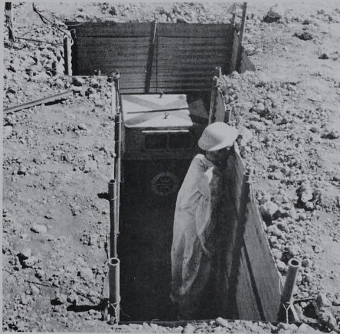
FIGURE 23. DUMMY IN TRENCH AT 2390 ft BEFORE FIRING
